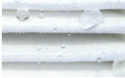
The NanoPleat filter material proven in long-term water test.
